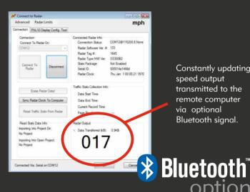
Constantly updating speed output transmitted to the remote computer via optional Bluetooth signal.
